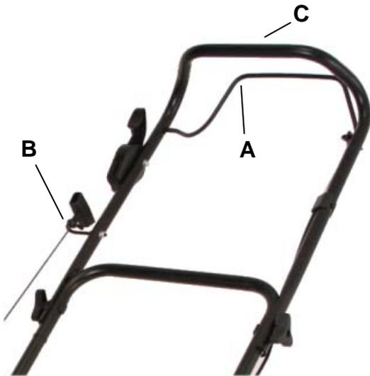
Pull the handle (A), that releases the brake for the knife towards the steering handle (C), and pull the starting cord (B), so that the cord may be placed into the holder.
